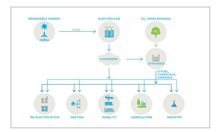
Figure 2. Overview of the P2X process <sup>3</sup>
