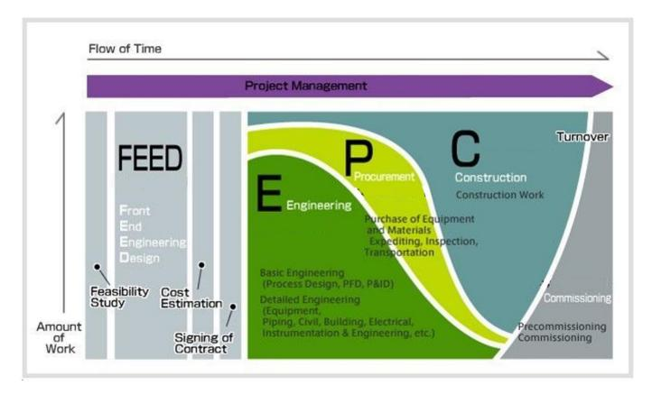
Figure 3. Overview of the EPC project model <sup>5</sup>
